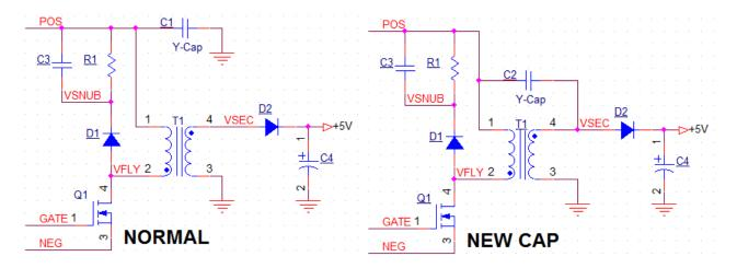
In its simplest implementation on a typical single positive output flyback supply (see above), simply remove the existing "normal" Y-cap and add a "new" Y-cap connecting a primary common to the other end of the secondary winding which is traditionally connected to the output diode anode (see above). This forces the inverted secondary voltage through the "new" Y-cap applying it in series with the leakage capacitance causing the opposing currents to cancel.
