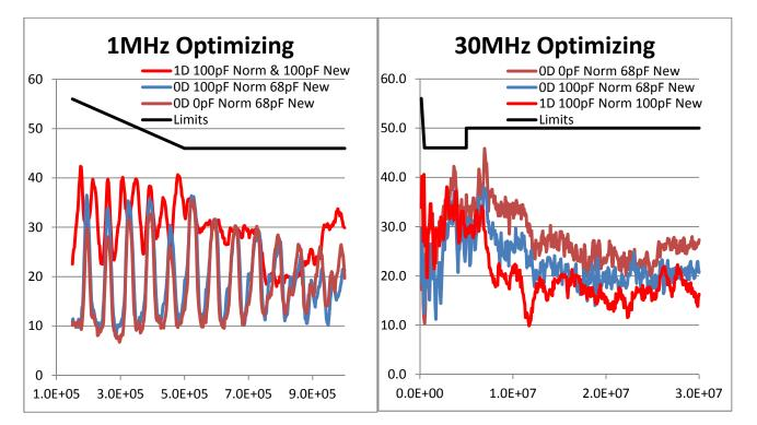
Also of note, the 100pF "normal" capacitor may be omitted if there is enough margin. Adding or omitting the diode or "normal" Y-cap may change the "new" capacitor value a bit. In my actual implementation, the optimum value changed between 68pF and 100pF. Either way, the optimum value should be established by experimentation. If the transformer construction changes afterwards, the optimum value should be verified and possibly reestablished.
